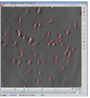
The goal in setting these three parameters is to make the cells bright compared to their background on the reconstructed image.
